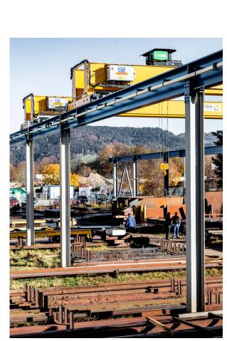
To cope with the increase in the volume and weight of material handled, the crane system in the storage yard of Stahlbau Schauenberg GmbH in Kirchzarten in southern Baden, Germany, was modernised with two double girder overhead travelling cranes with a span of 20 metres and a lifting capacity of 10 tons each.
